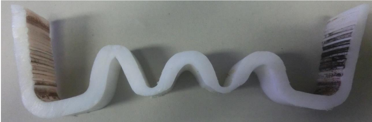
Fig. 2: Poor shaping of the PTFE bellows with extreme wall thickness variation
